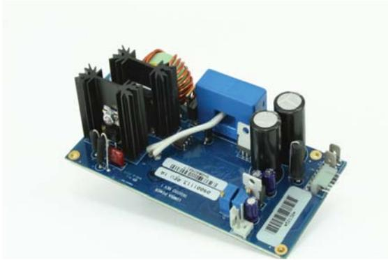
The LDPC series laser diode drivers offer the laser designer a compact low cost power supply for a variety of medical and industrial applications. In order to take full advantage of this unique product, care must be taken during the design process to ensure long term reliability. These application notes include answers to many commonly asked questions about the various configurations available and includes critical cooling and electrical information.
